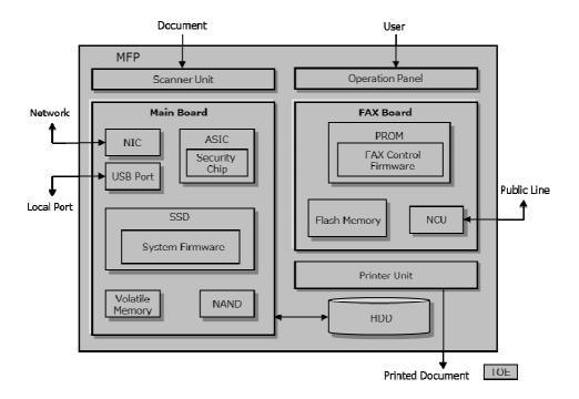
The Operation Panel is the hardware that displays status and results upon receipt of input by the TOE user. The Scanner and Printer units are the hardware that input documents into the TOE and output documents as printed material.
